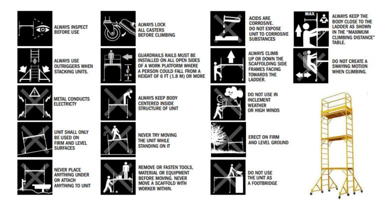
Follow the manufacturer's allowable load for the casters, scaffold components and platforms, along with recommended bracing to ensure a rigid and structurally sound scaffold.
